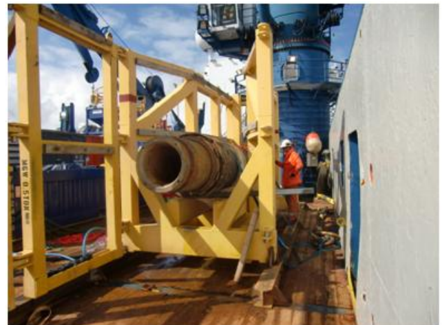
Wellhead in NCA purpose built landing frame for safe landing of wellheads on the vessel deck.
