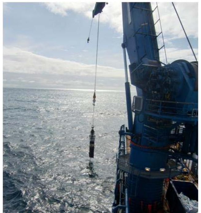
Recovery of wellhead using the active heave compensated crane on MSV Geosund
