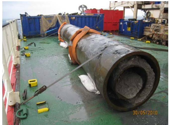
Recovered wellhead secured on deck of MSV Seawell
