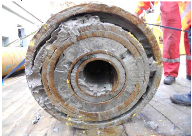
Cut profile of 15/22-5 (cut through pin and box of 20in connector)
